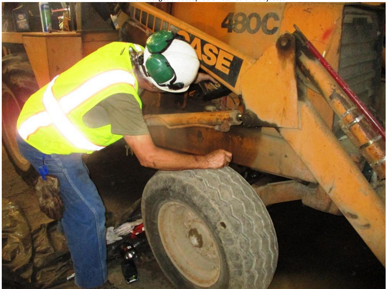
After installing a new hose for the power-steering fluid, Ed fills the back-hoe with said fluid
