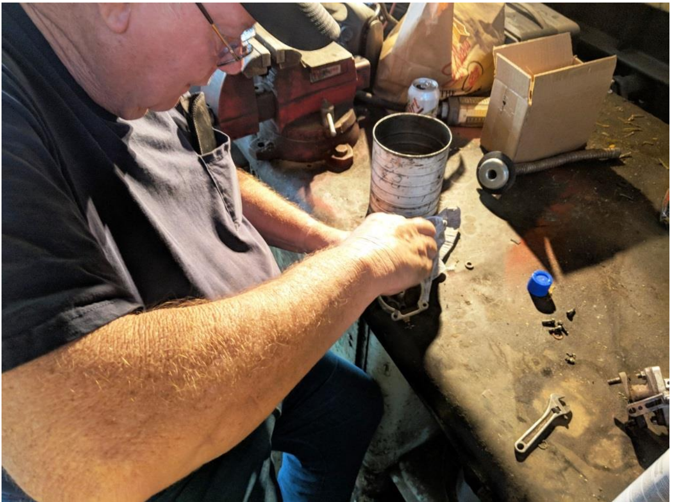
Gene rebuilds the A-5 motorcar's carburetor
