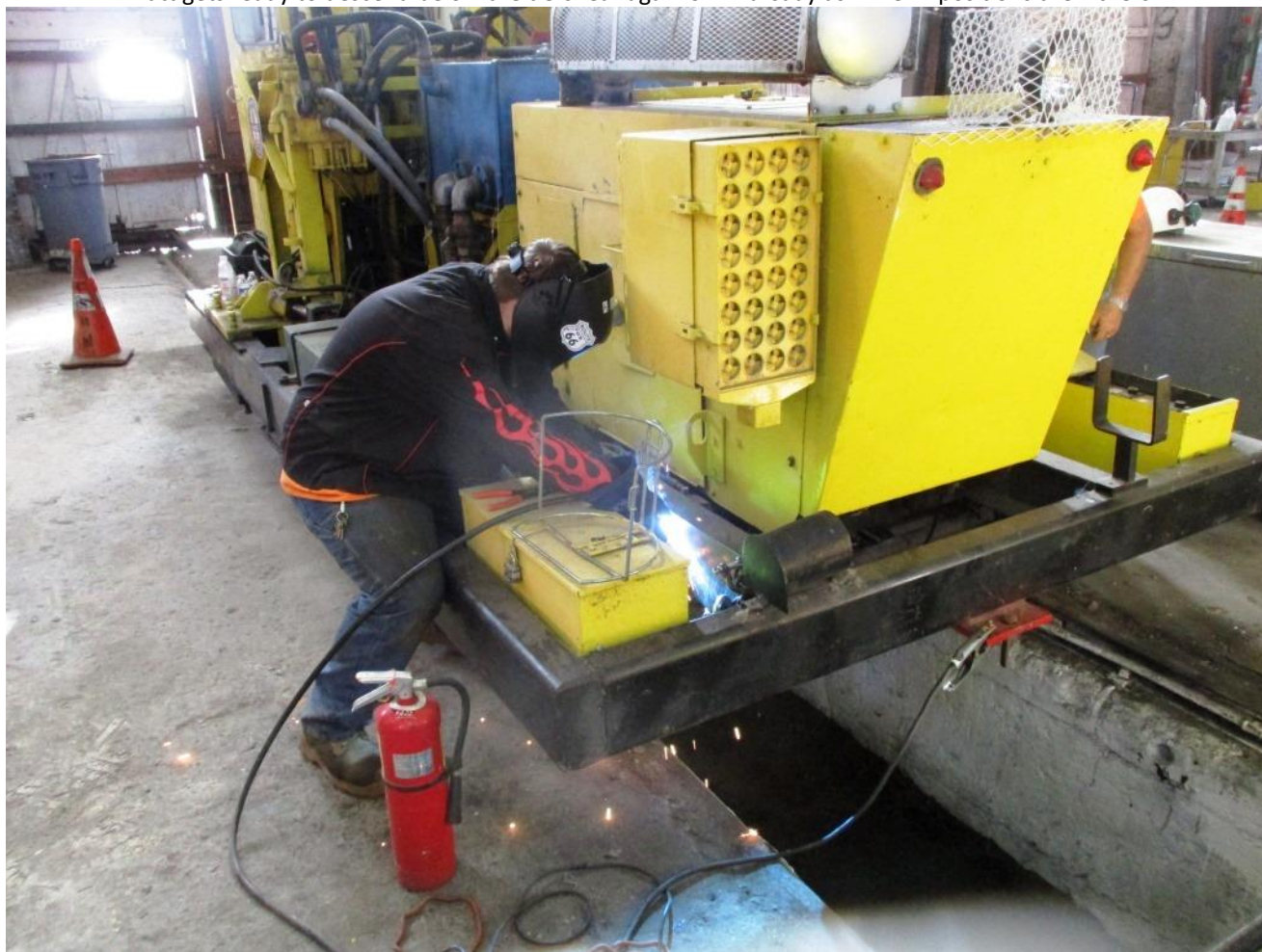
Chris welds the derail wheel's securing-chain back in place
